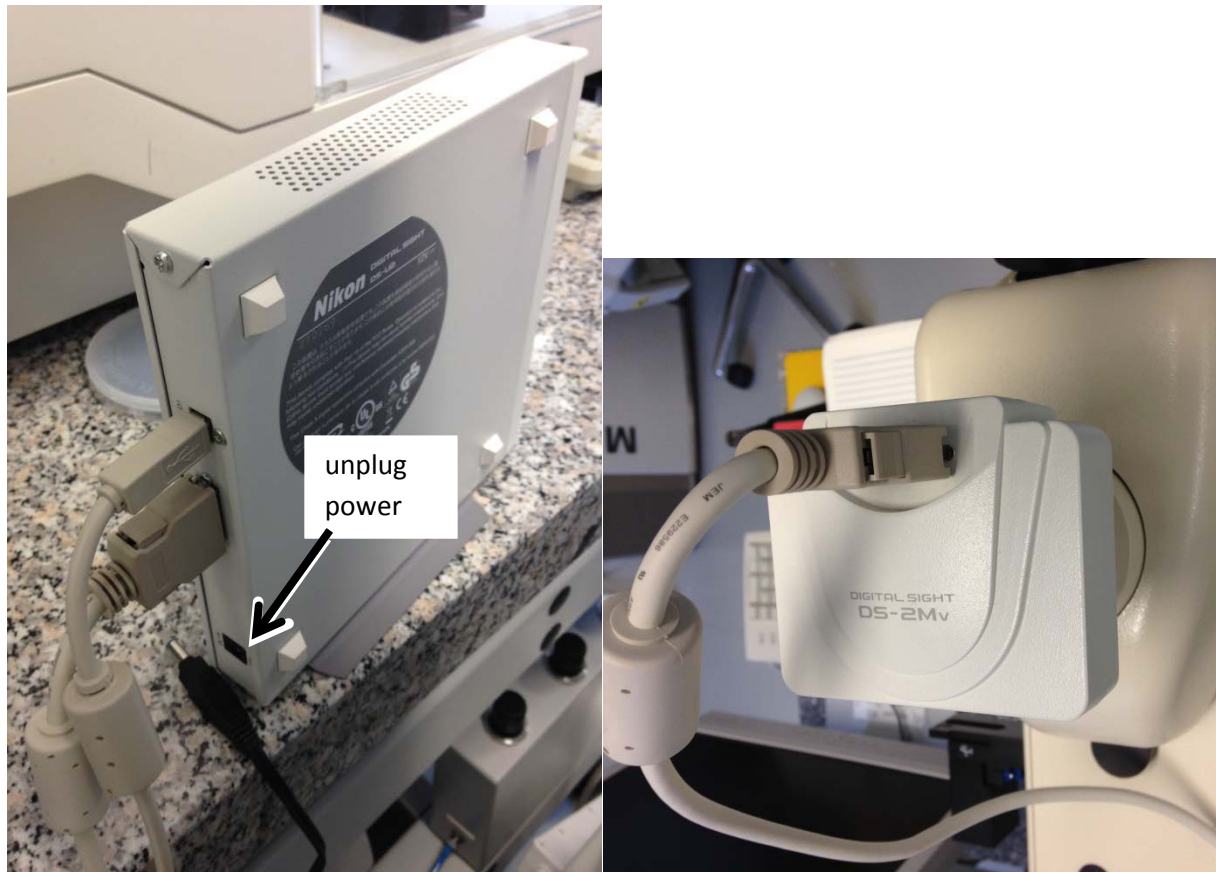
Fig 2: usb box: digital sight DS-U2 , Camera box with lense: digital sight DS-2Mv ; serial number 201115
